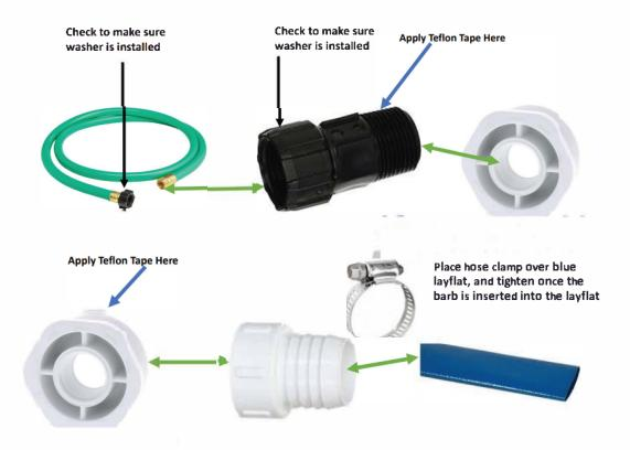
If you have trouble inserting the fitting into the blue lay flat, try adding a little olive oil to the first few ridges on the barb
